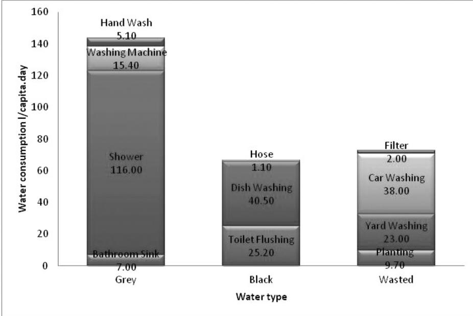
Fig. 2. Plumbing fixtures classified according to end water type.
