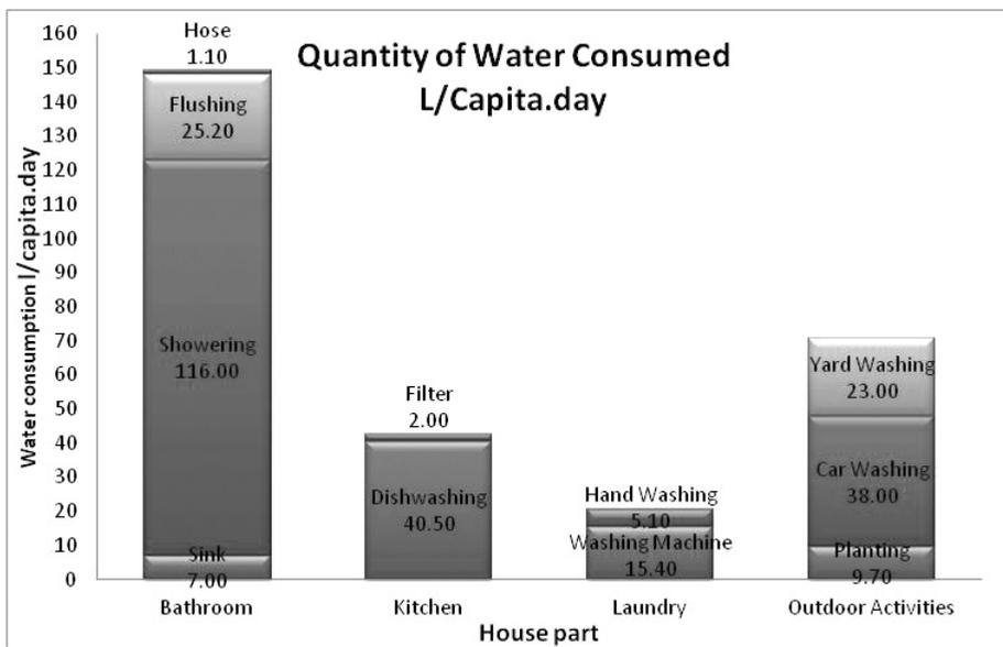
Fig. 1. Quantity of water consumed for different plumbing fixtures.
